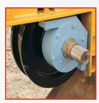
Wheel assemblies : Long travel wheels are straight treaded double flanged forged steel wheels. Wheels are supported on antifriction ball or double row self aligned spherical roller bearings in special blocks of 'L' type design ('I' type bearings) for easy maintenance.
